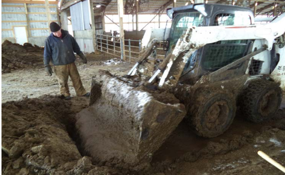
Photo 1 – A skid loader scrapes manure from the barn alleys into collection gutters
